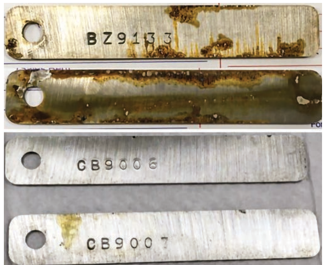
FIG. 3. MS coupons before (top) and after.
