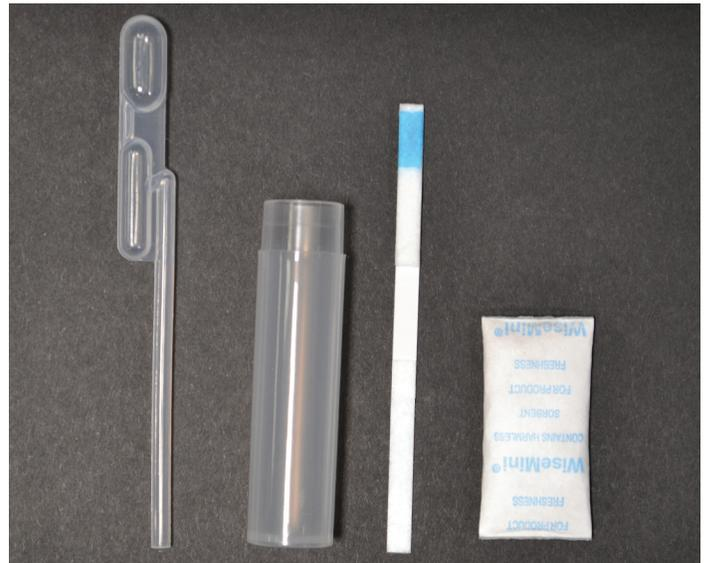
Test kit components (from left to right): volumetric pipette, test vial, test strip, desiccant
